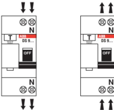
*Power supply can be connected to the circuit breaker from either upstream or downstream, without any difference.*
